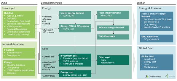
Figure 37. BEP tool calculation procedure
