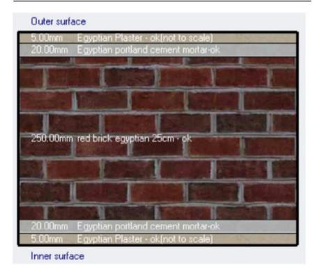
Figure 13. External walls main characteristics and U-values in residential buildings in Egypt (Fahmy, Mahdy, Rizk, & F. Abdelaleem, 2018)
