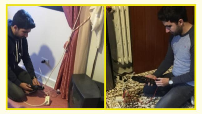
Figure 7 The on-site survey included a visual check of the appliances and their power rating as well as measurement of their actual consumption
