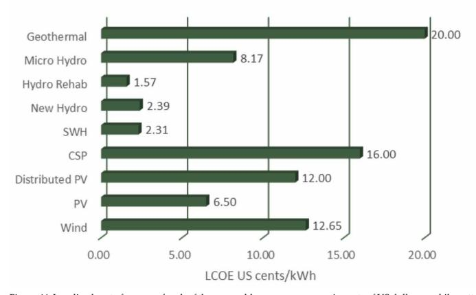
Figure 44. Levelized cost of energy of each of the renewable energy resources in cents of US dollars per kilowatthour
