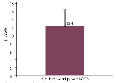
Figure 12. Levelized cost of wind power from onshore wind
