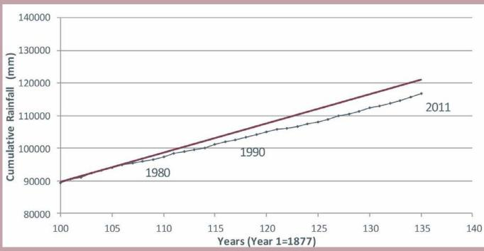
Figure 28. Cumulative rainfall in Beirut for the period 1877 to 2011. Schéma Directeur Hydro-Electrique au Liban, by Sogreah-Artelia, 2012, Beirut, Lebanon: Ministry of Energy and Water. Copyright 2012 by Ministry of Energy and Water.
