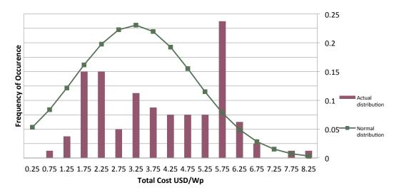
Figure 17. Price distribution for distributed solar PV based on NEEREA implemented projects
