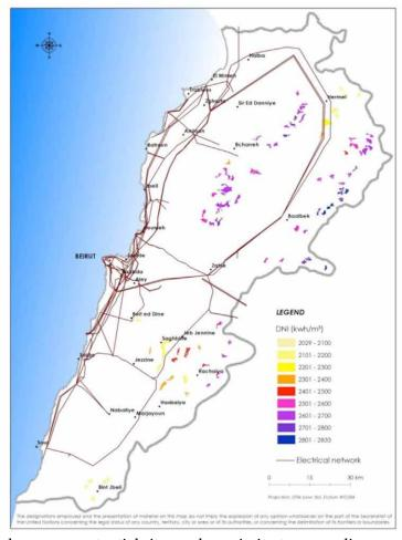
Figure 20. Concentrated solar power potential sites and proximity to power line
