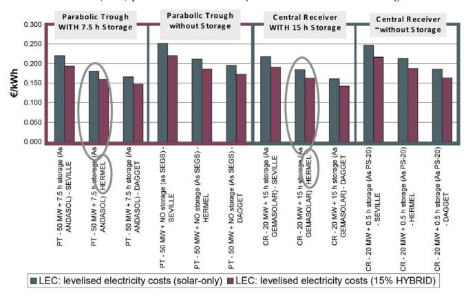
Figure 21. Levelized electricity costs for the 12 concentrated solar power potential sites in Lebanon (UNDP-CEDRO, 2012)
