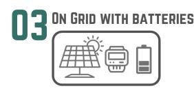
Also known as dual mode systems, these combine the features of on grid and off grid systems: they are connected to the grid and include batteries for storage.
