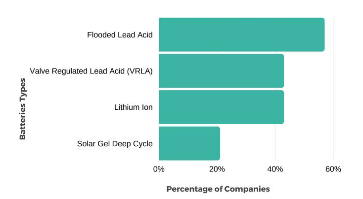
The graph above shows the distribution of batteries types employed by the participating solar PV suppliers in Lebanon. The most common battery type is the **Flooded Lead Acid** accommodated by 58% of respondents. **Valve Regulated Lead Acid (VRLA)** and **Lithium Ion** batteries are used by 43% of respondents each, while **Solar Gel Deep Cycle** batteries are employed by 21% of respondents in their installations.
